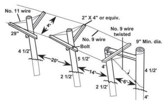
Figure 1. Details for the double curtain trellis.
