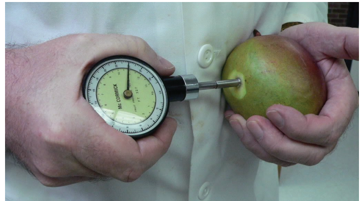
Figure 42. Measuring firmness with a handheld penetrometer.
