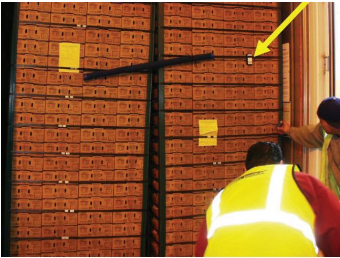
Figure 9. A portable temperature recorder on a load of mangos. Credits: J. K. Brecht, UF/IFAS
