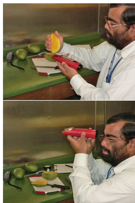
Figure 34. Measuring mango fruit SSC with a refractometer.
