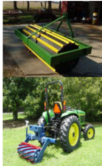
Figure 4. Roller-crimpers designed to terminate cover crops for reduced tillage systems. Top: Roller-crimper designed by D. Treadwell and M. Alligood, Horticultural Sciences Department, University of Florida 2006. Bottom: Roller-crimper designed by R. Raper, USDA-ARS-NSDL Conservation Systems Research, Auburn, AL Credits: Top: D Treadwell. Bottom: R. Raper
