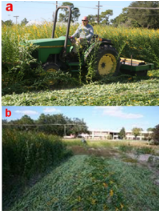
Figure 3. A) Roller-crimper designed by Alligood and Treadwell, terminating sunn hemp in Gainesville, FL, at mid-bloom. B) Terminated sunn hemp immediately following rolling and crimping. Credits: D. Treadwell
