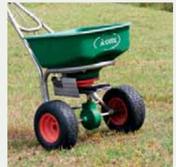
A deflector shield directs fertilizer away from your maintenance-free zone.
