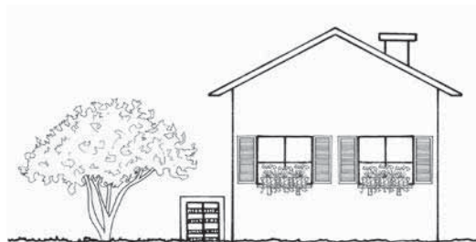
Shade your A/C unit from direct sun, but do not block the airflow.
