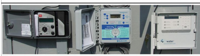
Figure 1. Photo of three brands of ET controllers from testing at the University of Florida, Agricultural and Biological Engineering Department.
