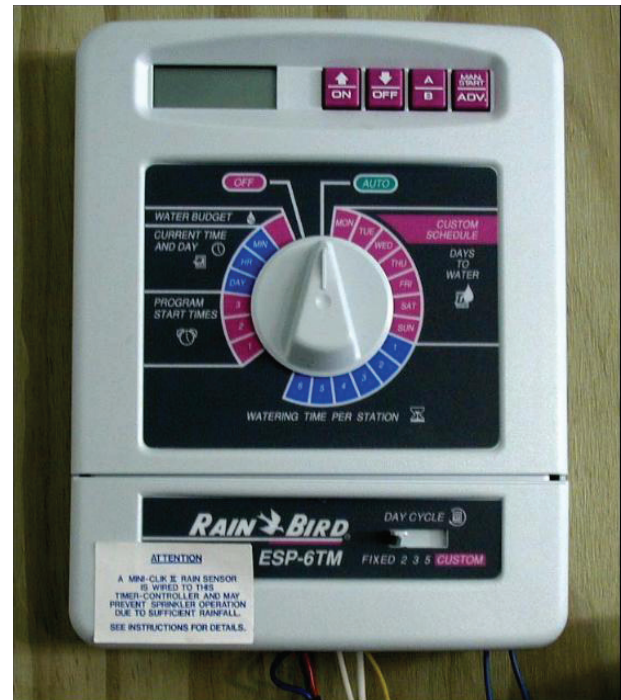
Figure 1. Typical residential irrigation controller.
