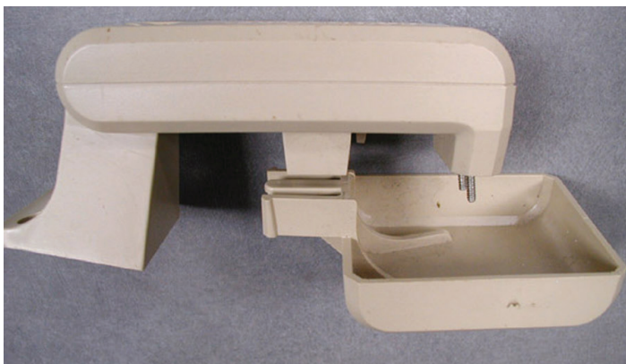
Figure 2. Hygroscopic shutoff device based on electrical conductivity.
