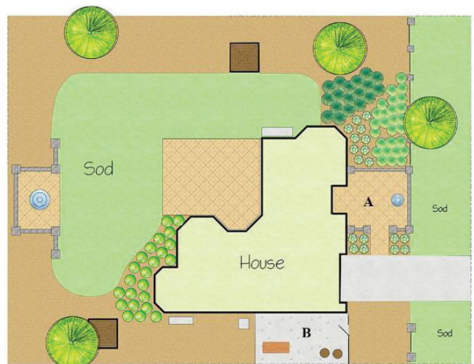
Figure 18. Install hard surfaces, such as patios or courtyards, before adding new plant material.
