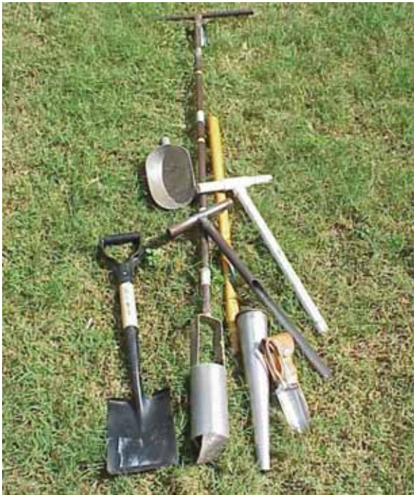
Figure 6. The collection of soil samples for nematode analysis can be acquired from the field using either cylindrical sampling tubes, trowels, bucket auger, or shovel.
