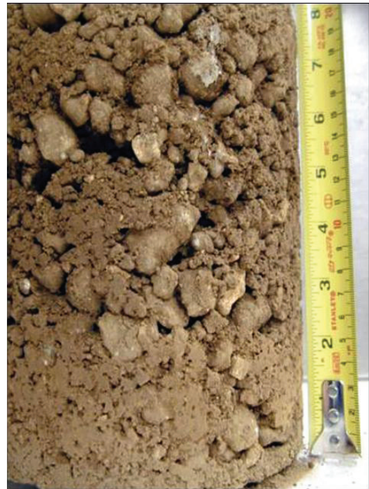
Figure 4. The profile of a gravelly soil. The soil is typical of soils found in the Homestead area, in the southern peninsula of Florida. Credits: R. Muñoz-Carpena, UF/IFAS
